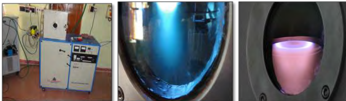
Photograph of Sputtering facility at Nano Markers, Photograph of Sputtering –Ar plasma, Ar +N 2 plasma
